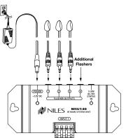
Figure 5: Connection Ports
